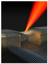
strain landscape induced in the atomically thin semiconductor leads to the formation of a potential well, where single-photon emitters are localized with a precision better than 140 nm. Due to the elongation of the well either along or across the rod axis, the polarization of the emission is found to be oriented in the respective two directions.
