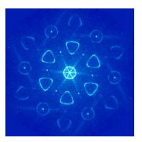
a drastic change in the QPI, indicating a state with broken chirality. Two effects are driving this transition: First, the trigonal warping of the constant energy contour opens up a new scattering channel. Second, higher order electron hopping pushes the Van Hove singularity down to lower energies.
