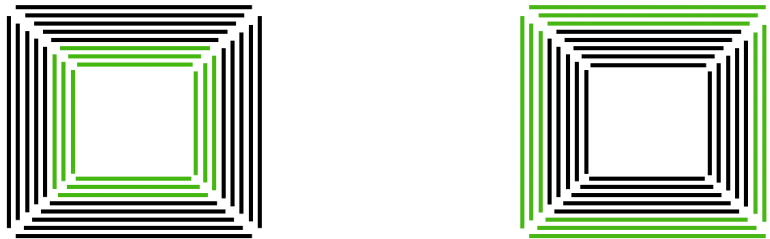
Fig. X.4: Module selection used for the qualitative non-collinearity model comparison. Simulations were made for all modules whereby only coincidences from the highlighted modules (lime-green) were accepted. In detail, only the innermost three or outermost three modules were used.
