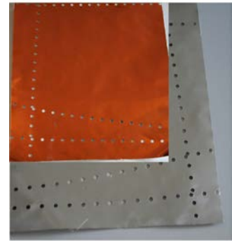
Fig. V.14: Rotating stamp perforation of lead-Kapton samples performed by Schober. The diameter of the holes was 4 mm.
