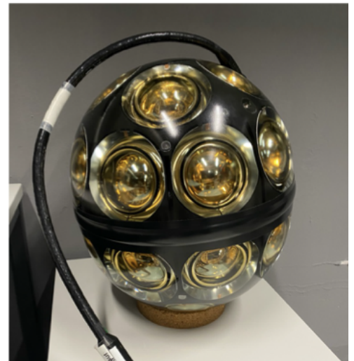
Figure 2.7: Picture of an mDOM. The yellow-tinted components are the 24 PMTs.
