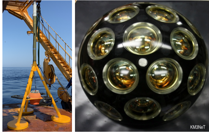
Figure 3.2: Left: Acoustic emitter (white) on a tripod right before deployment. Picture: KM3NeT collaboration. Right: Picture of a DOM with a piezo sensor. The device is glued directly to the glass sphere. From [48], p. 8
