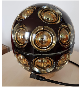
FIGURE 2.3.1: Photo of a Prototype of an mDOM, one of the IceCube Upgrade's new optical modules. Taken from [12].
