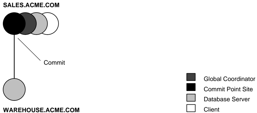
Figure 3-4 Determining the Commit Point Site
