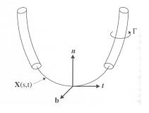
$$egin{aligned} & ' \equiv rac{\partial}{\partial s} \ & \text{Curvature } \kappa = rac{\| ec{t}' \|}{\| ec{t} \|}, \ \kappa = rac{1}{R} \ & \text{Torsion } au = rac{ec{b} \cdot ec{n}'}{\| ec{X}' \|} = rac{ec{X}' imes ec{X}'' \cdot ec{X}'''}{\| ec{X}' imes ec{X}'' \|} \end{aligned}$$
