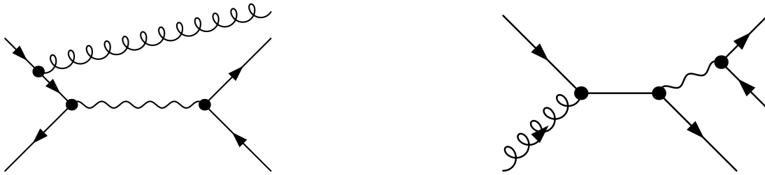
Figure 2.4: Real correction contributions for the \mathcal{O}(\alpha_s\alpha) contribution to the NLO Drell-Yan cross section. In addition, there is a u-channel for the quark emission and similar antiquark emission diagrams.
