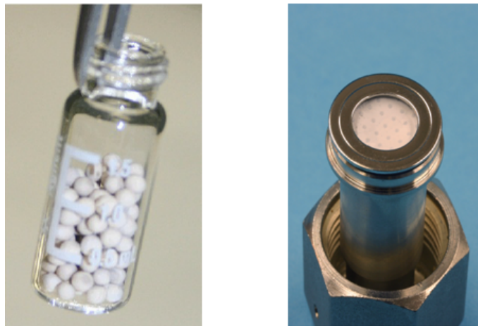
Figure 9: Left: ^{83}\text{Rb} source embedded in zeolite pellets[Han2011]. Right: Top of the rubidium source with the protective PTFE membrane filter[Ave2012].
