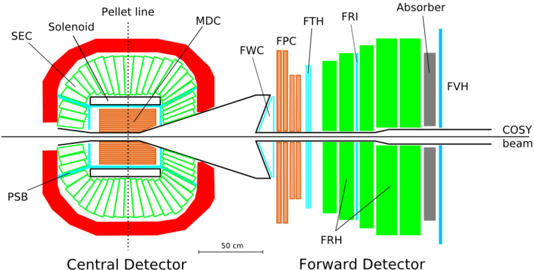
$^3\text{He}$  detected in Forward Detector
